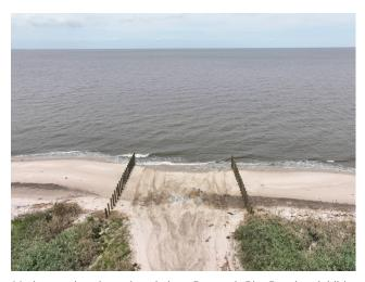
Marine-grade pylons placed along Bennett's Pier Beach to inhibit vehicle trespass.
